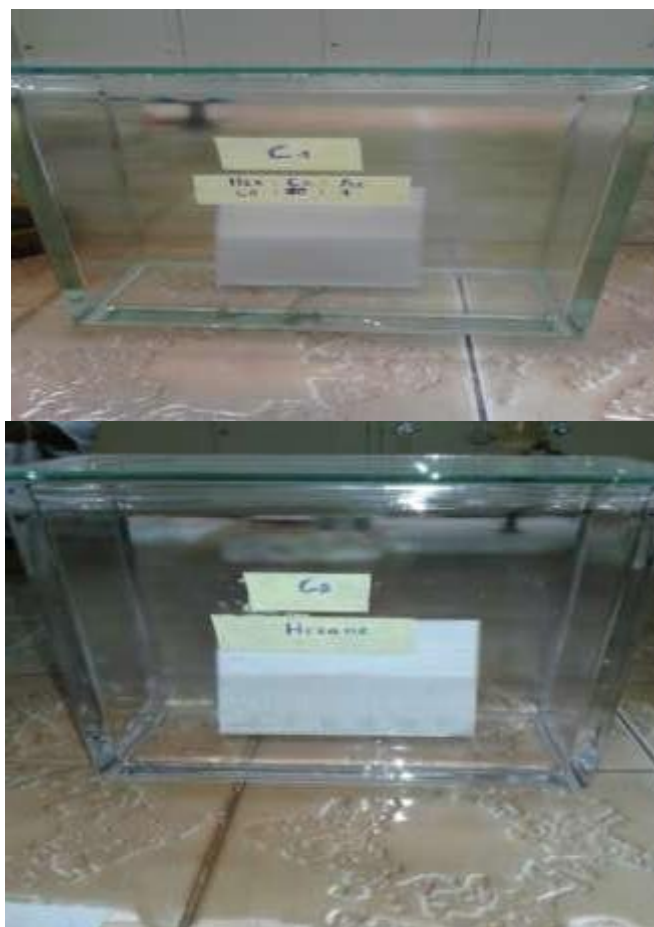
Figure 19: Photographs showing a first eluting in hexane: ethyl ether: glacial acetic acid (40: 10: 1 v / v / v) up to half of the plate (left) and a second elution in hexane until a cm from the upper edge of the plate (right).
