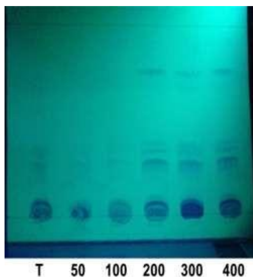
Figure 22: Picture of the plate with UV 254 nm before revelation with \text{CuSO}_4 II, showing the migration of different neutral lipids. (Photo of Oluwagbemiga Amos S., 2015)
